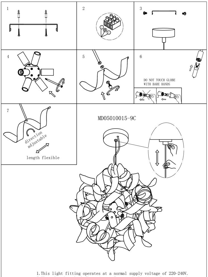
1. This light fitting operates at a normal supply voltage of 220-240V. 2. When changing the bulb or fuses, always switch off at the mains and allow the old bulb to cool down before handling.
