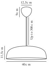
Voltage (V): 220-240 Volt IP degree: IP20 Maximum bulb wattage (W): 3\*25 Class (Class 1, Class 2, Class 3): Class 2 (Double isolated) Socket type: E14 Parallel connection: False
