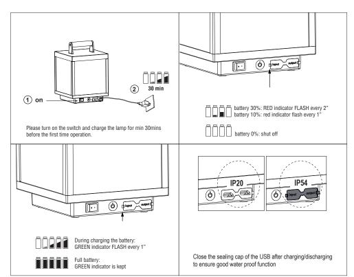
NOTE: It will dim off the lamp and no dimming when charging, also no discharging function in this situation; Never short circuit the imput and output of the lamp, or pls restart the lamp with switch.
