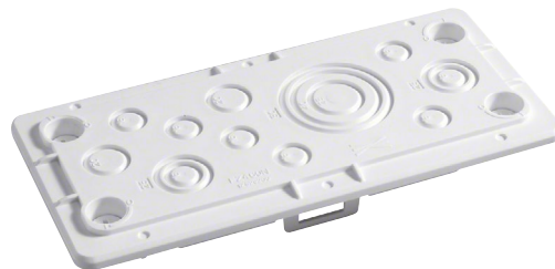
FZ460N cable entry with pre-stamps 6xM16, 2xM20, 2xM16/25, 1xM25/40/50
