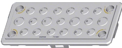
FZ466N cable entry with pre-stamps 15xM16 and 4xM20
