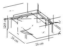
Voltage (V): 220-240 Volt IP degree: IP44 Maximum bulb wattage (W): 15W Class (Class 1, Class 2, Class 3): Class 2 (Double isolated) Socket type: E27 Parallel connection: True
