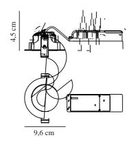
Voltage (V): 220-240 Volt IP degree: IP44 Class (Class 1, Class 2, Class 3): Class 2 (Double isolated) Socket type: LED Module Parallel connection: True
