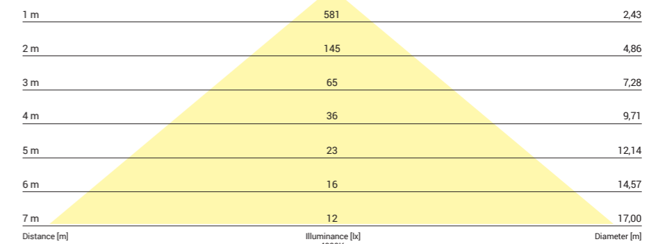
Beam cone diagram Beam angle 100°
