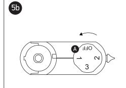
Circuit 2: Rotate the knob (A) 90° anti-clockwise from the starting position OFF, to connect circuit 2.
