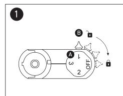
To mount the track adaptor into the track system, first check that the selector knob (A) is at OFF position and the adaptor lock **B** is disengaged.
