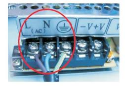
Connect the wires of the power adapter.
