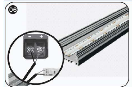
06 Connect strip wires to the output terminal of power supply, and dispose with waterproof, insulation, short-circuit and anti-corrosion protection at both the wire joints and the cut section of your strip (if any)
