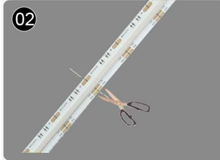
02 Calculate the needed length and cut off the extra length along cutting mark if necessary; if need to add wires, please weld them at the next location with printed mark.
